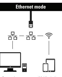
Capture images from any remote PC or Mac with access to your LAN network. Mobile devices can also be used, if they have access to your network ia Wi-Fi.
