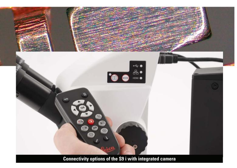
Use **USB mode** to connect the camera directly with a **PC** or Mac **via USB2** cable.
