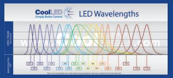
20 different LED wavelengths from the near-UV at 365 nm to the near-IR at 770 nm
