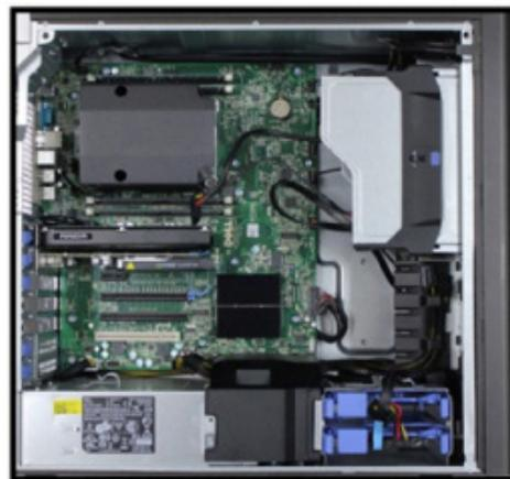
4. Locate an available 4 channel or higher PCIe slot (marked x4). Refer to the PC's documentation to locate a suitable slot.
