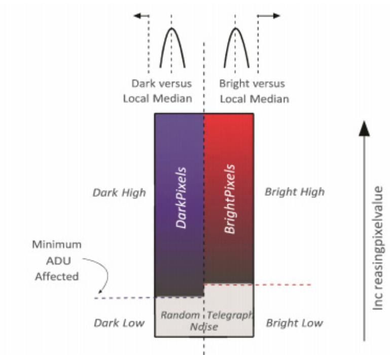
**Figure 8: Pixel Noise Filter**
